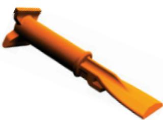
The Spartan™ Capping Removal Tool is a multi-purpose tool designed for the removal of capping, cleaning concrete from sideform and capping, and its unique ball lock rail base helps remove concrete build up. The Capping Removal Tool's molded ball lock rail base also helps pull sideform away from the finished concrete panel.
