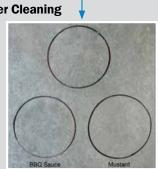
Testing was conducted on smooth, steel-troweled concrete test specimens. Concrete test specimens were pre-treated with **Duro-Nox** liquid silicate floor hardener. The pre-treated test specimens were then treated with two coats each of the stain protectants (Duro-Guard or **Duro-Polish Plus**), applied in accordance with the recommended application guidelines.
